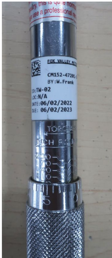
A calibration certification label is meaningless if the wrench has been dropped or abused.
