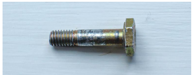
This bolt was "screwed" into its hole, damaging the grip and stripping away the cadmium plating, which protects the grip from corrosion.
