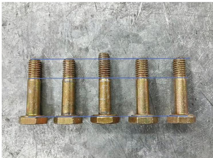
Variations in thread length can negate the rule of thumb that no more than three threads should protrude from a nut.
