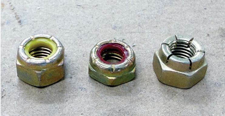
Stop (lock) nuts come in a few varieties. The most common are the AN365 elastic stop nut and the AN363 all-metal stop nut. A low-profile elastic stop nut – the AN364 – is also available.
