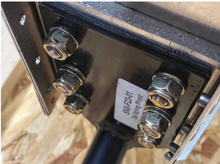
This is an abandoned Sonex project. Neither the hardware callouts in the plans nor best practices can explain why the builder placed two washers under each bolt head, leaving the nuts barely clinging to the threads.
