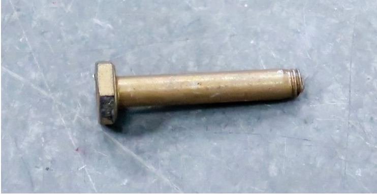
This bolt broke at the threads, which are not intended to carry shear loads.
