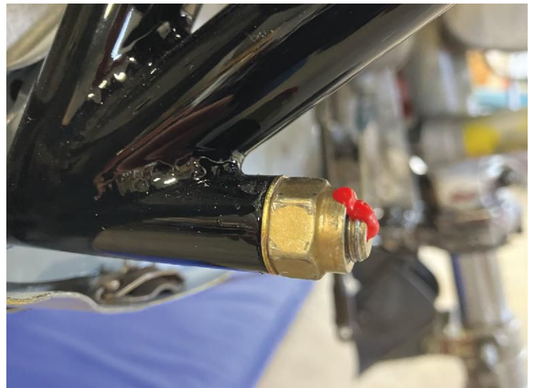
Torque seal will visually reveal if a nut has turned on the threads, but it will not reveal if embedding loss has occurred.
