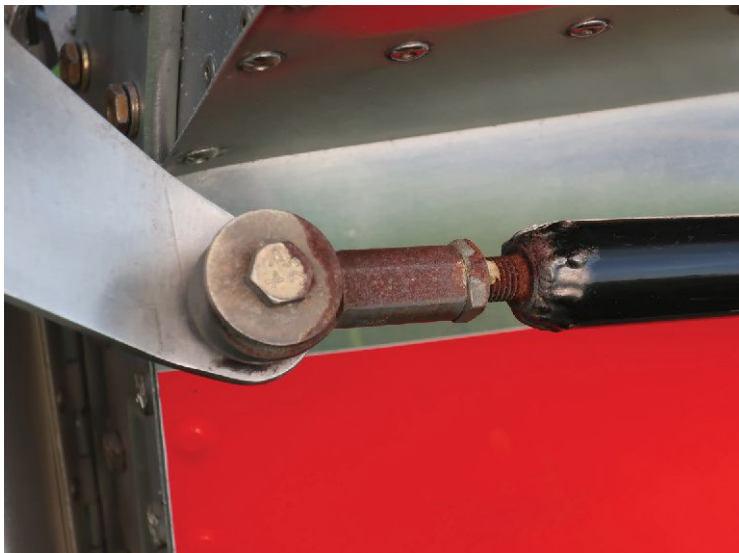
AN970 washers are larger in diameter than AN960 washers and must never be omitted when called for in construction documentation. They do critical work, like spreading loads across the surface of soft materials and capturing rod ends in the event of a failure.
