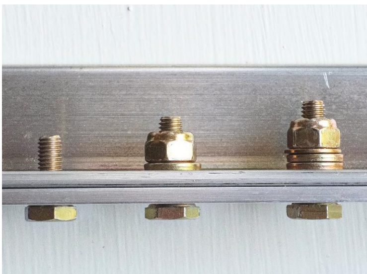
By observing how much grip extends through a hole, you can choose the correct bolt length. The bolt on the left is too short. Its grip is within the parts being fastened. The bolt in the middle is correct, its grip extends fully through the parts and one washer will prevent the nut from bottoming out on the grip. The bolt on the right is too long and would require too many washers.
